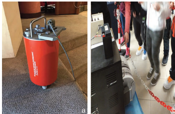
Figure 9 a) S-13 short-period seismometer (© Photo [5]); b) some students who simulate an earthquake by jumping all together in front of the seismometer.
