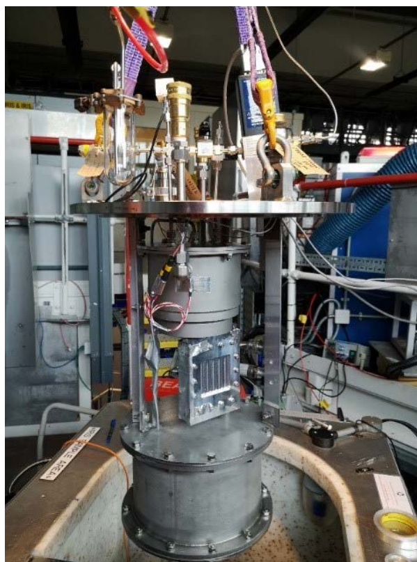
Figure 2 The \text{CO}_2 mineralization reactor rig being installed into the sample area of the IRIS beamline at RAL-ISIS. The rig position is adjusted such that the sample cell is aligned with the neutron beam (N) ( Rev. Sci. Instrum. , 2023, 94 , 093905).
