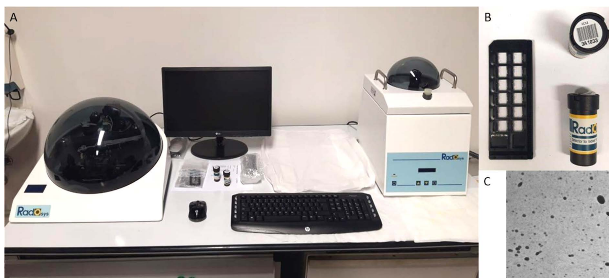
Figure 1 RADOSYS system used at the INGV Radionuclides laboratory (A) to perform analyzes on passive nuclear track detectors (CR-39) (B). Track-etch that are used in exposures for prolonged periods (months), as indicated by the European directive 2013/59 Euratom dated 5/12/2013. Computerized analysis of CR-39 by electron microscope for automatic detection of traces and obtaining the average indoor radon concentration during the exposure period (C).
