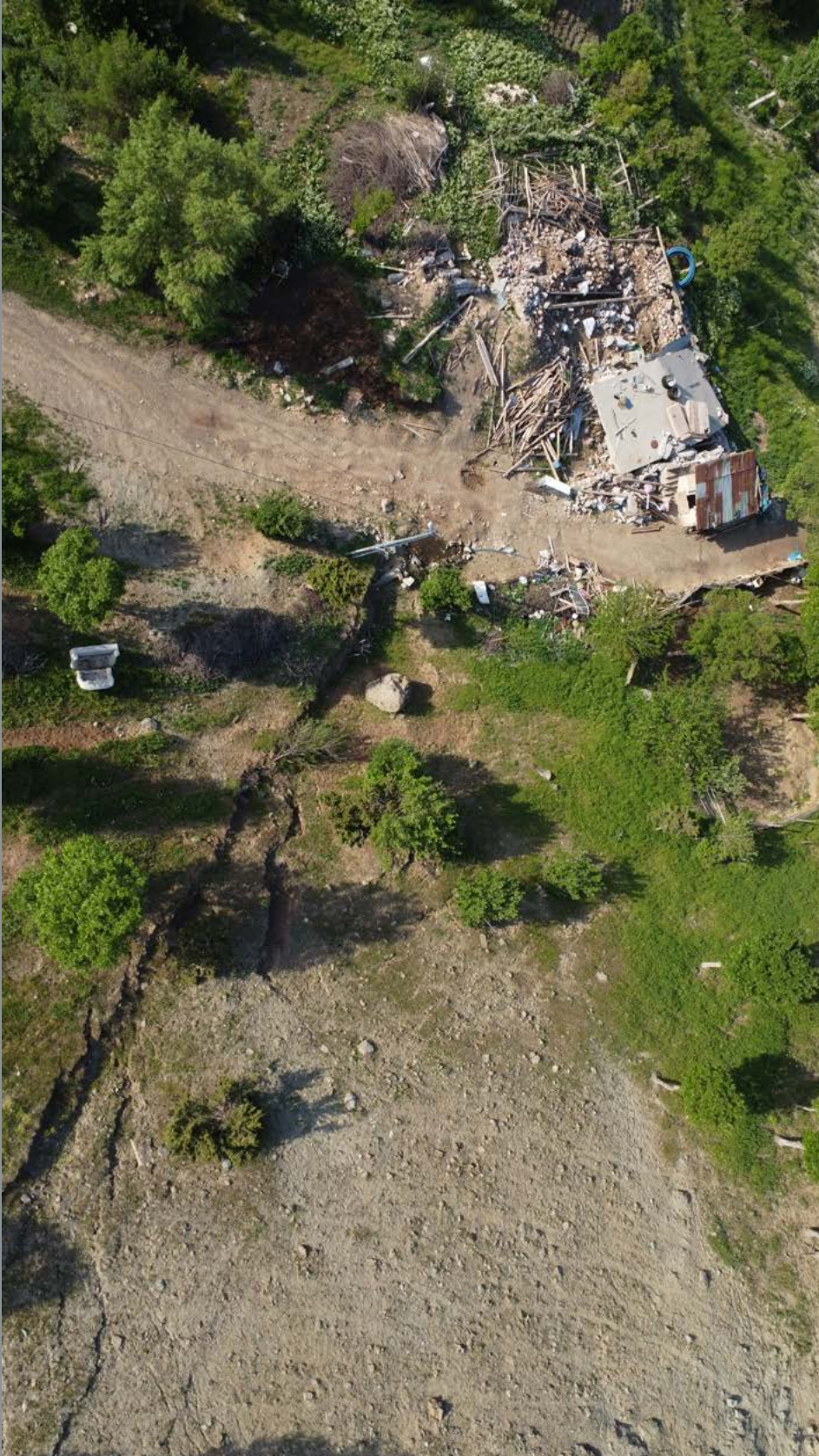
Photo 77 (37.619174°N, 37.387709°E) – Azimuthal view of the coseismic rupture crossing a farm and causing its complete collapse.
