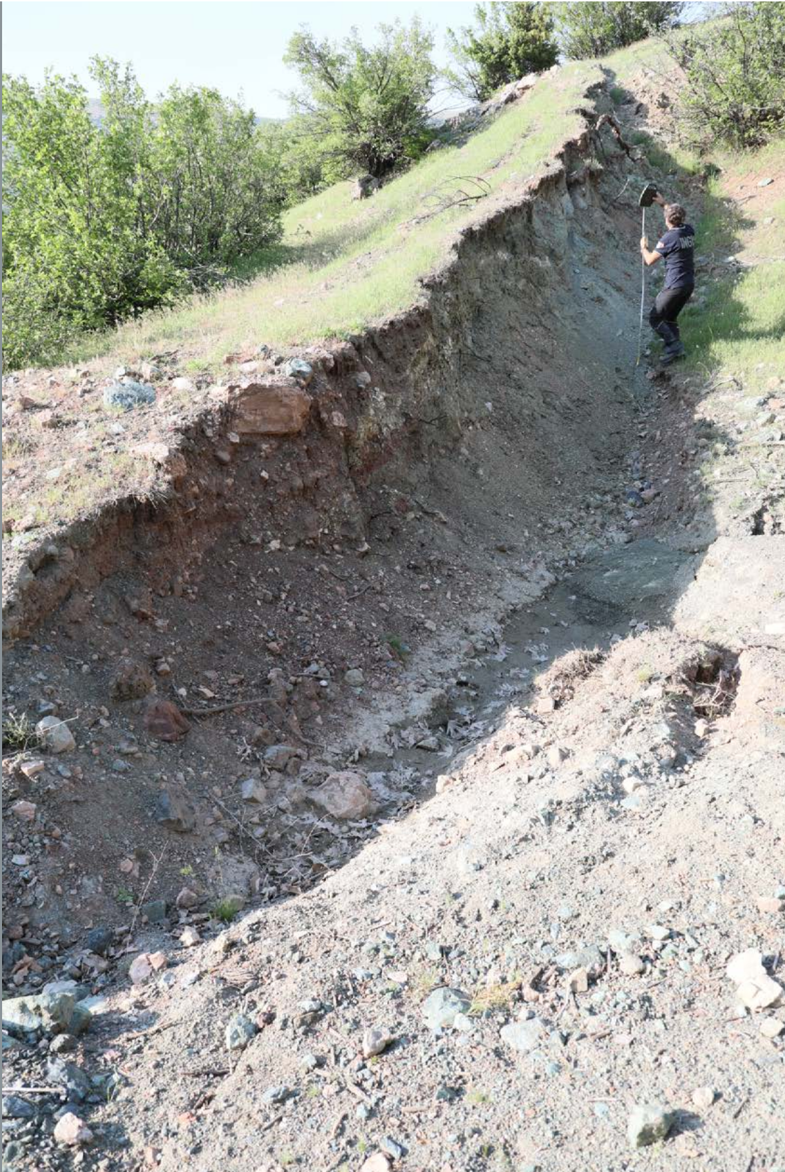
Photo 57 (37.615527°N, 37.383265°E) – The apparent vertical offset component of up to 210 cm is given by the lateral dislocation of the oblique slope.
