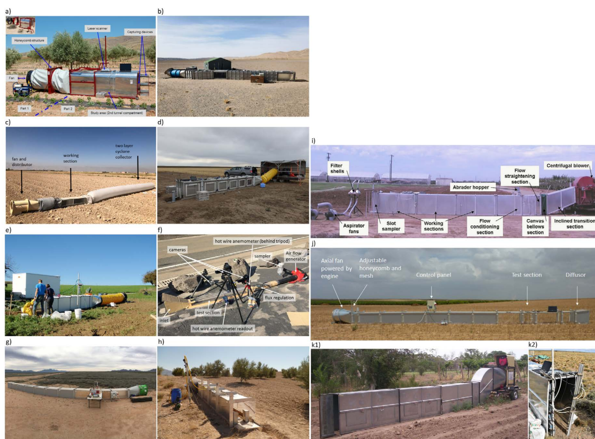
Figure 13 Aerodynamic configurations and velocity profiles in portable tunnels. This figure illustrates the technical differences between the suction and blowing systems used in in situ experiments. The plots highlight the development of the boundary layer within the tunnel, which is crucial for ensuring that wind simulations accurately reflect natural conditions and for precisely determining the sediment detachment threshold across different soil types.
