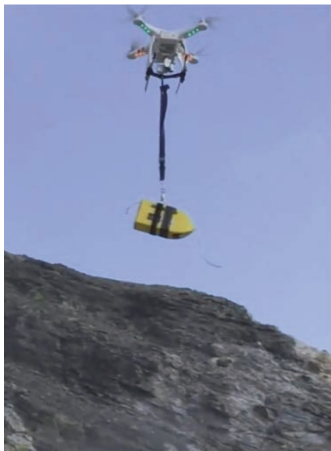
Figure 3 MiniGas Dragon - UAV Test Unit mounted on DJI Phatom Vision 2 Quadcopter . Figura 3 MiniGas Dragon - UAV Test Unit istallato sul DJI Phatom Vision 2 Quadcopter .
