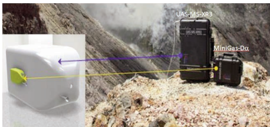
Figure 2 UAV-MS-XR3 Mass Spectrometer for multiple gas analysis and MiniGas payload (UAS airborne configuration in left, ground test units on right).
