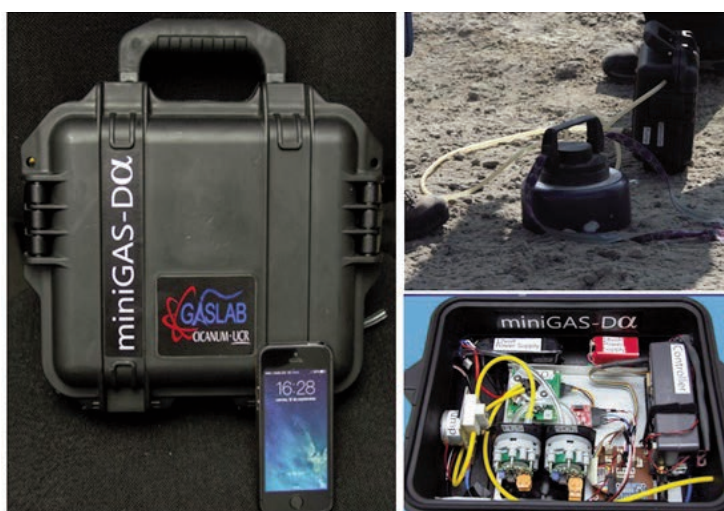
Figure 1 MiniGas D α Field Test Unit for CO 2 , SO 2 e H 2 S, T, P, RH and GPS telemetered in situ measurements.
