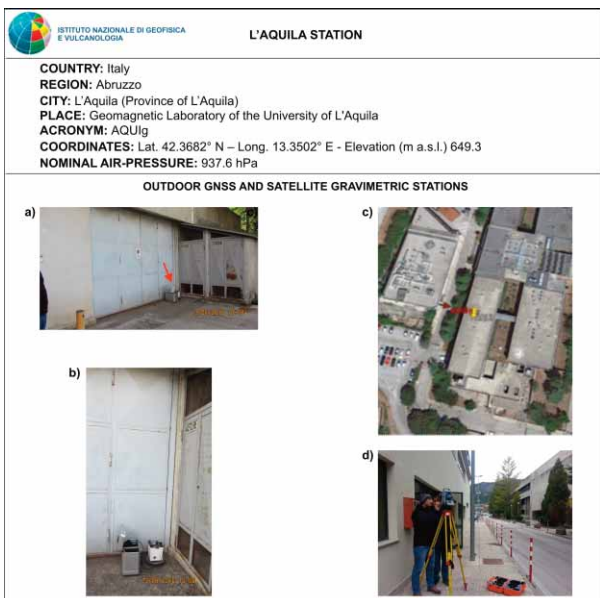
Figure 4b Schematic monograph and photos of L'Aquila (AQUlg) satellite gravity and GNSS (AQUI) stations. a) and b) location of the outdoor satellite gravity station with the exact position of the relative gravimeter LCR-D#85; c) location of the GNSS station (AQUI) settled on the roof-top terrace of the building; d) topographic measurements to connect the outdoor station AQUl with the indoor absolute station (AQUlg; see [Fortunato et al., 2020]).
