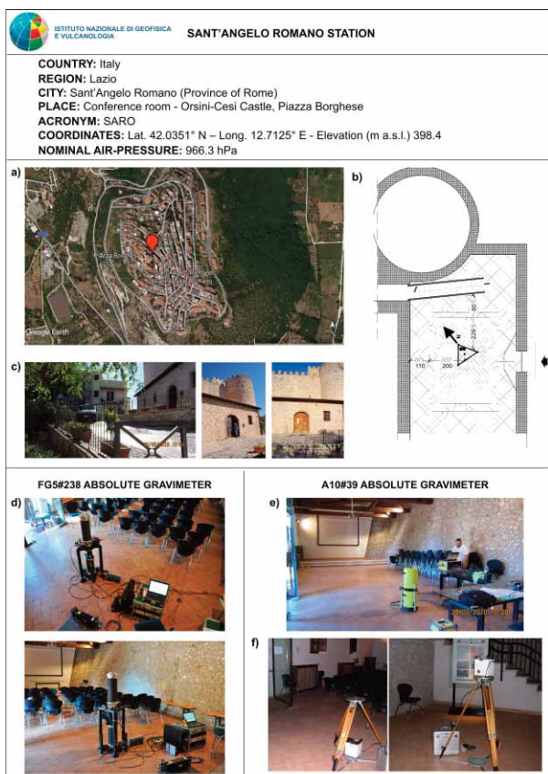
Figure 2a Schematic monograph and pictures of Sant'Angelo Romano (SARO) absolute gravity station. a) Google Earth view of Sant'Angelo Romano village where the Orsini-Cesi castle is located; b) map of the conference room with the exact location of the measurement point; c) photos of the exterior of the castle showing the entrance of the conference room; d) and e) the Micro-g LaCoste FG5#238 and A10#39 during the measurement sessions, respectively; f) the supports to measure the vertical gravity gradient at different heights with the relative gravimeter LCR-D#85.
