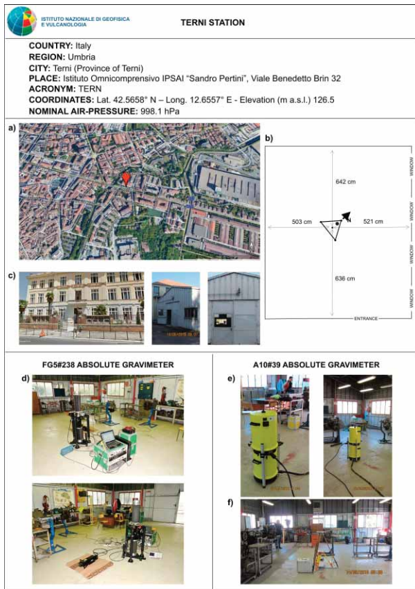
Figure 5a Schematic monograph and photos of Terni (TERN) absolute gravity station. a) Google Earth view of the Istituto Omnicomprensivo IPSAI “Sandro Pertini”, located in Viale B. Brin 32, in the city of Terni, selected to make the absolute gravity measurement; b) map of the Officina n. 4 with the exact location of the measurement point; c) exterior of the school and the main entrance of the Officina Motori n. 4; d) and e) the Micro-g LaCoste FG5#238 and A10#39 during the measurement sessions, respectively; f) the supports to measure the vertical gravity gradient.
