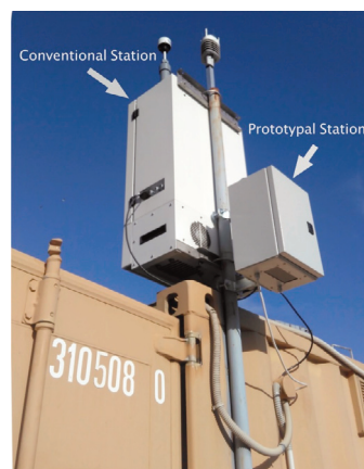
Figure 6b Back-to-back installation of the conventional station (AQM-65) and of the prototypal station both mounted on an Iso 20' container.
