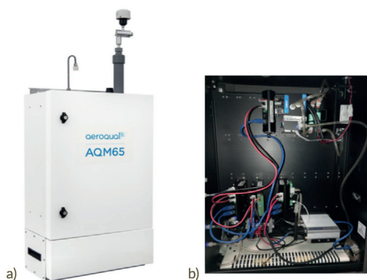
Figure 1 a) Commercial monitoring station (mod. Aeroqual - AQM65); b) Installed sensor modules, cooling system (on the bottom), data transmission and embedded mini-pc.
