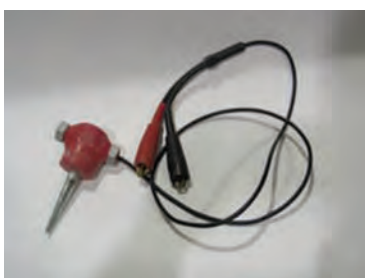
Figura 33 Sismometro Mark L-15B a componente verticale ( www.ce.unlv.edu/egl/Equipment ). Figure 33 Vertical component Mark L-15B seismometer ( www.ce.unlv.edu/egl/Equipment ).
