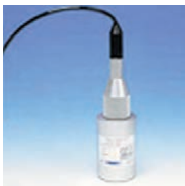
Figura 32 Sismometro Mark L4-C a componente verticale ( www.sercel.com ). Figure 32 Vertical component Mark L4-C seismometer ( www.sercel.com ).
