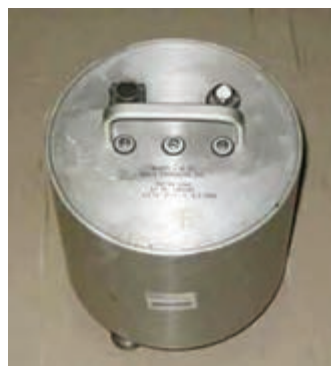
Figura 34 Sismometro a tre componenti Mark L4-3D ( www.ija.csic.es ). Figure 34 Three-component Mark L4-3D seismometer ( www.ija.csic.es ).
