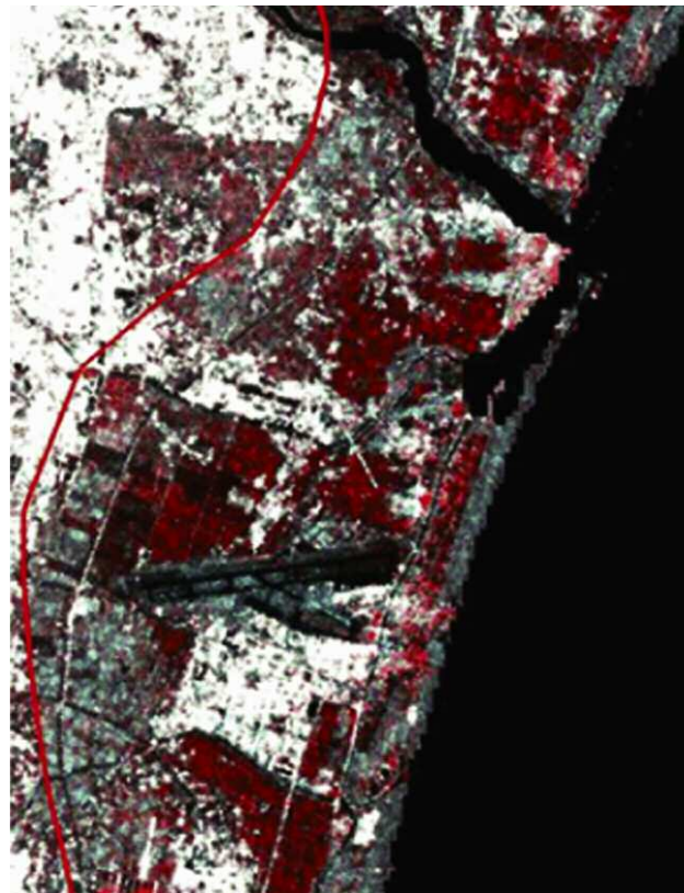
Figure 27 RGB color composite of two SAR backscattering images (R: 19/02/2011; G: 21/03/2011; B: 21/03/2011). In red and cyan are highlighted the areas of changes. Red continuous line is the estimated inundation limit.
