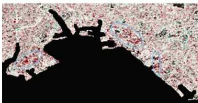
Figure 28 Upper panel shows a RGB color composite of two SAR coherence images, R=Pre-seismic (21/11/2010-19/02/2011); G=Co-seismic (19/02/2011-21/03/2011); B=Co-seismic (19/02/2011-21/03/2011); Lower panel shows a RGB color composite of two SAR intensity correlation images, R=Pre-seismic (21/11/2010-19/02/2011), G=Co-seismic (19/02/2011-21/03/2011); B=Co-seismic (19/02/2011-21/03/2011); the blue ellipses represent the decorrelation due to major surface liquefaction effects, which are in accordance with [Kishada, 2001].
