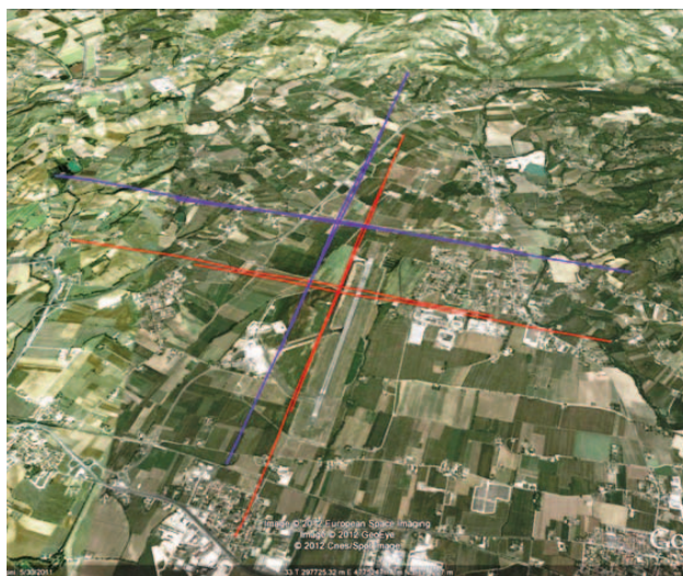
Figure 3 Calibration flight performed over the airport of Perugia on the 23th June 2012. The red flight lines are at an altitude of 700 m agl, the blue flight lines at 1400 m agl..
