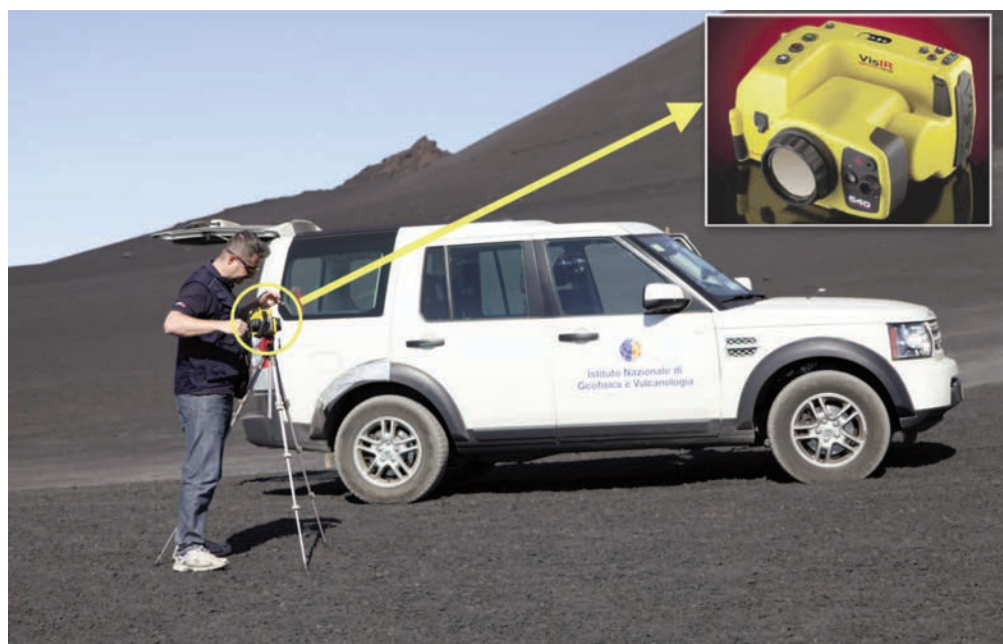
Figure 25 Thermal camera mounted on tripod. Figura 25 Camera termica montata sul treppiede.
