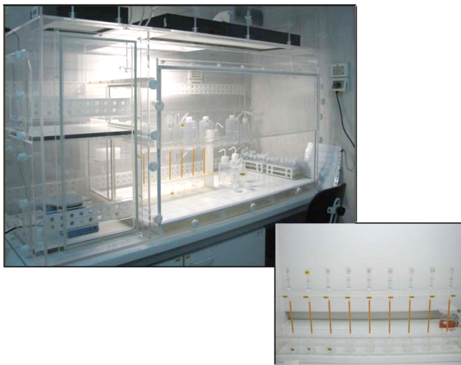
Figure 1. Detail of the quartz columns for Sr and REE separation by chromatographic techniques.
