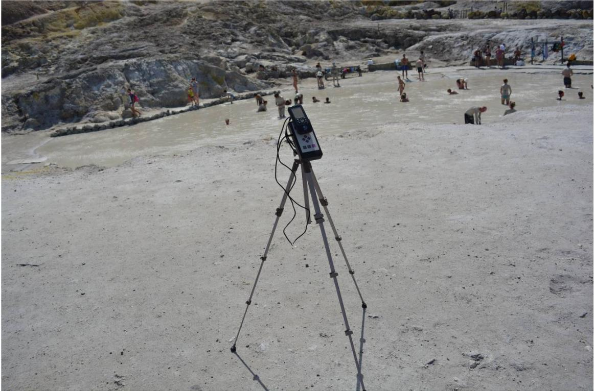
**Figure 22.** Microtops sun photometer mounted on its tripod with connected GPS.
