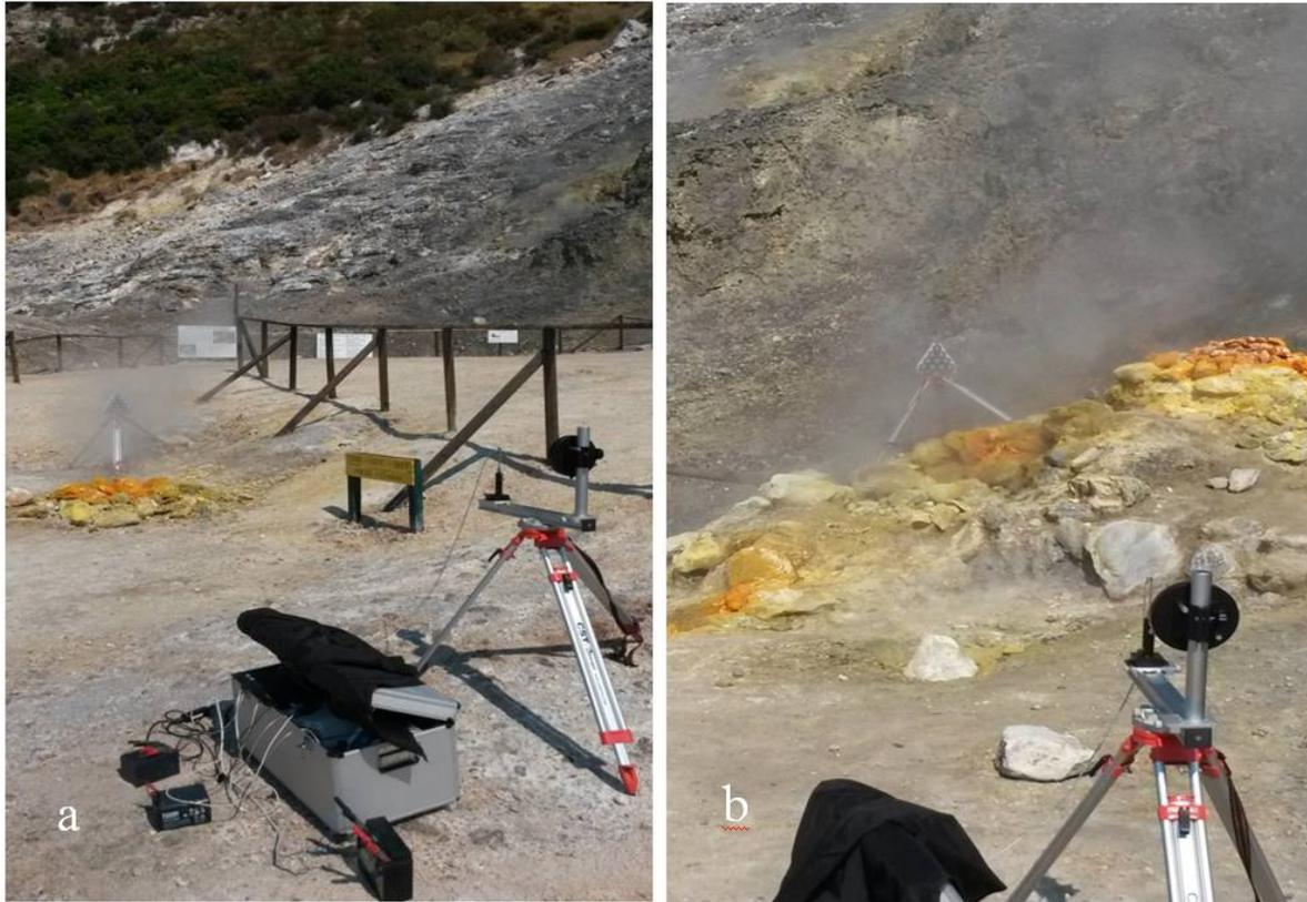
**Figure 20.** Location of the LP-DOAS during the measurement period at La Solfatara on September 01, 2015. The reflectors are placed directly behind a higher temperature fumaroles a) Bocca Nuova, b) Bocca Grande.
