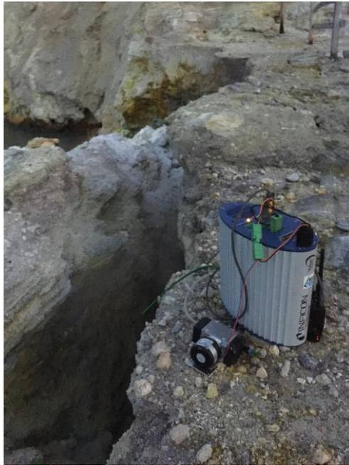
**Figure 1.** Vulcan T-Guard sensor, produced by INFICON.
