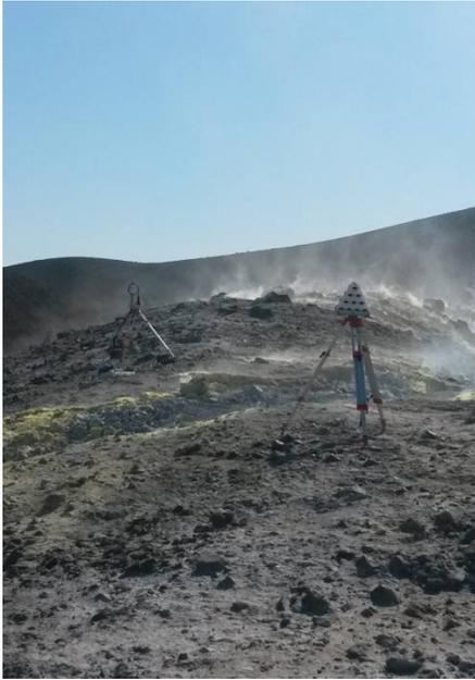
**Figure 21.** Photograph of the positioning of the Active-LP DOAS during the measurements made at Vulcano Island through the high temperature fumarole (F0).
