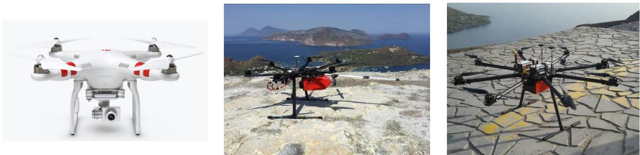
**Figure 15.** Drones used during the campaigns: DJI Phantom Vision 2 Quadcopter (left), DJI S800 Hexacopter (center), EPIC 8 Italdrone Octocopter (right).
