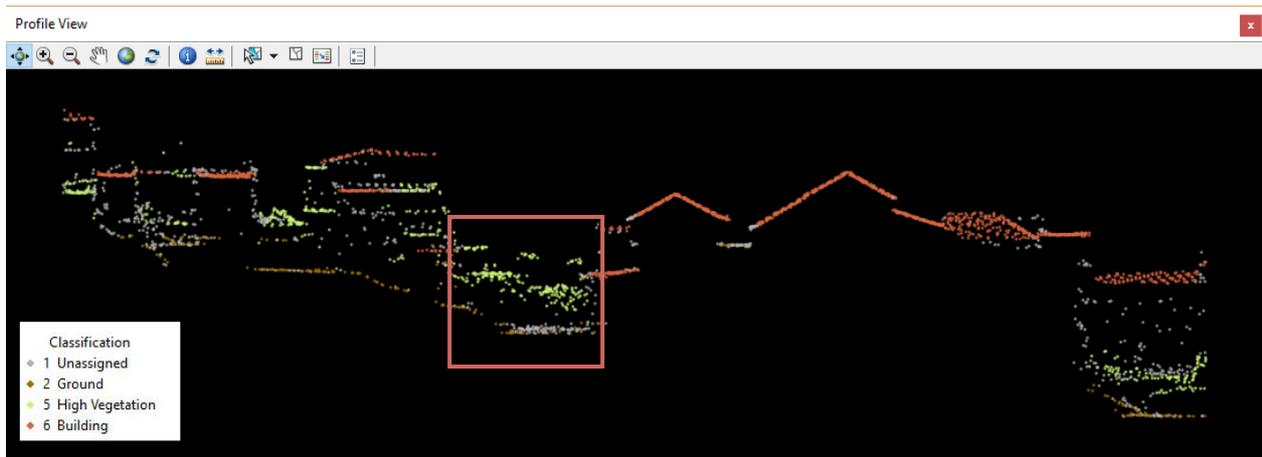
**Figure 10.** LiDAR points classification in densely urbanized area of Amalfi. The red box highlights a sector visible with greater detail in the next figure (figure 11).
