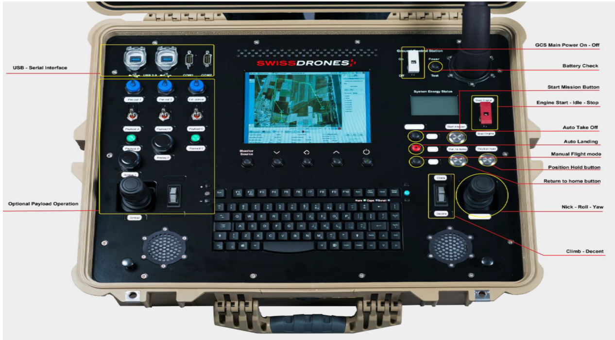
Figure 6. Ground Control Station (GCS) for UAV flight and mission control.
