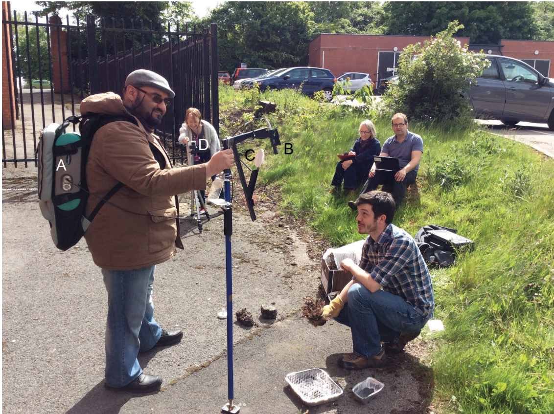
Figure 4. ASD Fieldspec FR (A) carried on back of operator, with the sensor head (B) and moveable white calibration panel (C) attached to a vertical pole. The TIR-VIS camera (D) is mounted on the tripod behind.
