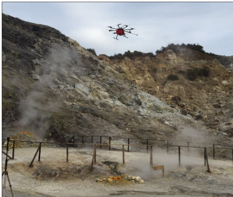
Figure 20. UAS-MiniMS-XPR3 flying over La Solfatara “Bocca Nuova” and “Bocca Grande” fumarole onboard INGV's Italdrone Octocopter.
