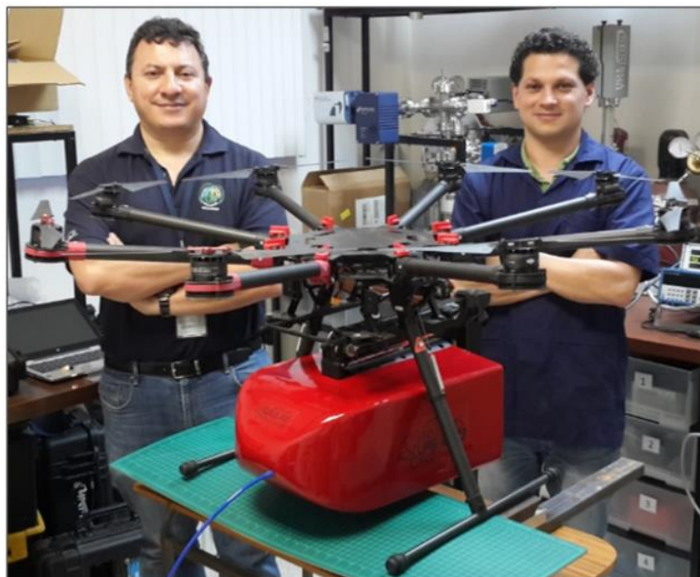
Figure 4. UAS-miniMS-XPR3 prototype integrated to S100+ drone for laboratory tests in Costa Rica.
