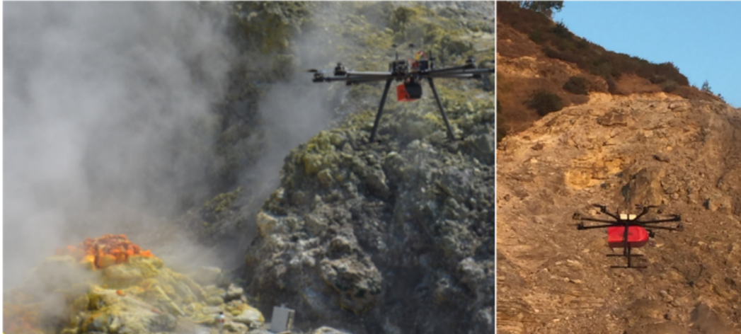
Figure 12. MiniGAS NTX (left) and UAS-miniMS XPR3 (right) mounted on E-EPIC 8 Italdrone Octocopter.
