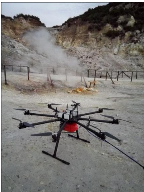
Figure 14. The NTX MiniGAS instrument integrated to Italdrone Octocopter at La Solfatara 2016 deployment.
