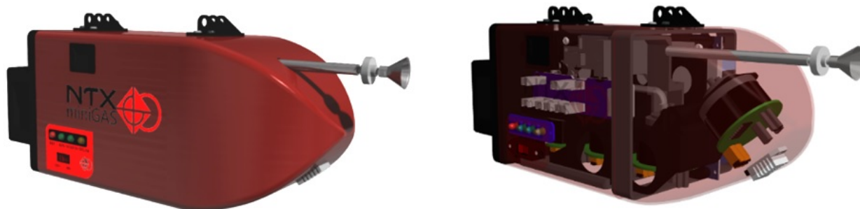
Figure 2. MiniGAS NTX System: Magmatic/Hydrothermal degassing monitoring payload for integration to unmanned aerial vehicles (UAV) and drones. System includes GPS based datalogger with telemetry for airborne, car or hand carried gas sampling, pressure, temperature, R= relative humidity and GPS sensors (T, P, RH% Lat., Long & Altitude); multiple single gas sensors: SO 2 , H 2 S, CO 2 . Onboard data logging (microSD card), telemetry, USB antenna receiver, software, external switchable power on/off, status LEDs, two hot-swappable power supplies capability, external anchor support. Payload system has been successfully tested in Kilauea, USA; Alaska, USA; Solfatara, Italy, Vulcano, Italy; Turrialba, Costa Rica; Poas Costa Rica; Masaya, Nicaragua. See following links:
