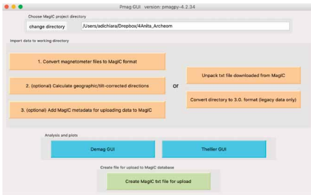
Figure 5 Example of the Pmag_GUI.py program, where one can change the working directory, import new data, convert them in a readable file and interpret them with Demag_GUI.py (for directional data) and Thellier_GUI.py (for intensity data).
