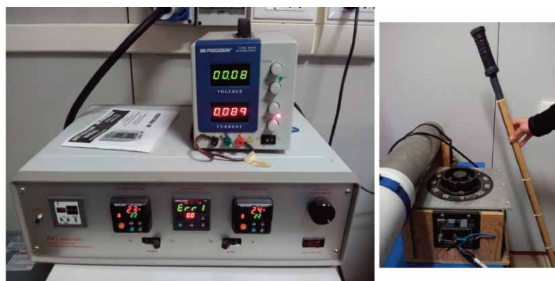
Figure 4 To the left, command panel to switch on the oven, control the temperature, regulate the timing for the fan. On top of the command box, there is the controller for the magnetic field inside the oven. To the right: variac to erase the residual field inside the oven. This step needs to be performed after each in-field step, Tx.1 o Tx.2, before a zero-field step, Tx.0.
