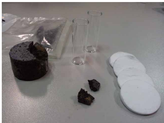
Figure 2 Standard paleomagnetic sample (cylinders with 2.5 cm in diameter and 2.2 cm high), fragments cut from it, glass filters and vials (not marked in the picture).
