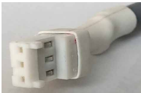
Figura 5 Connettore per DS18B20. Figure 5 Connector for DS18B20.
