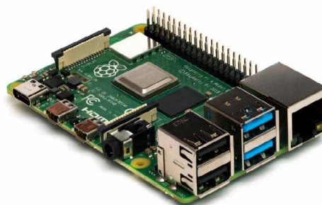
Figura 6 Raspberry Pi model B. Figure 6 Raspberry Pi model B.
