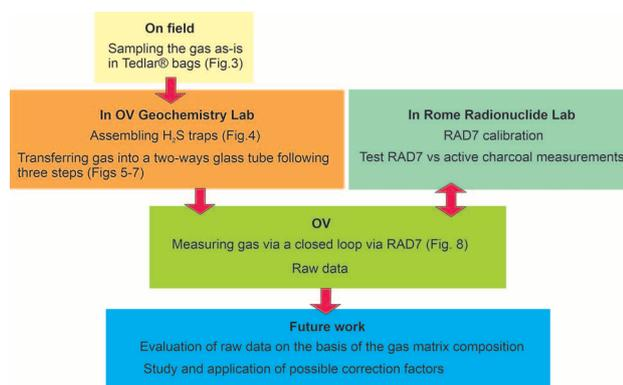
Figure 2 Steps in the proper-designed method for Rn measurement in gas fumaroles.
