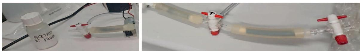
**Figure 4** H<sub>2</sub>S traps, made of lead acetate powder filled into silicone tubes. Note the colour of the traps: darkish on the right one due to the interaction with H<sub>2</sub>S from the incoming gas, and whitish on the left one after complete hydrogen sulphide removal.
