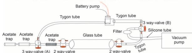
**Figure 5** 1<sup>st</sup> step: configuration for the glass tube to be under vacuum. On the right the vacuum rotary pump needed to create vacuum in the glass tube.
