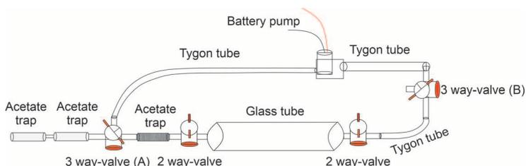
**Figure 7** 3<sup>rd</sup> step: scheme showing the configuration before measurement at RAD7. Note the A and B valves closed.
