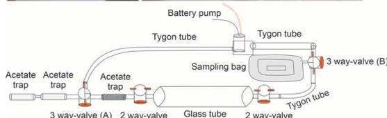
**Figure 6** 2<sup>nd</sup> step: gas transfer from the Tedlar® bag to the glass tube. Note the A valve closed towards the external way.
