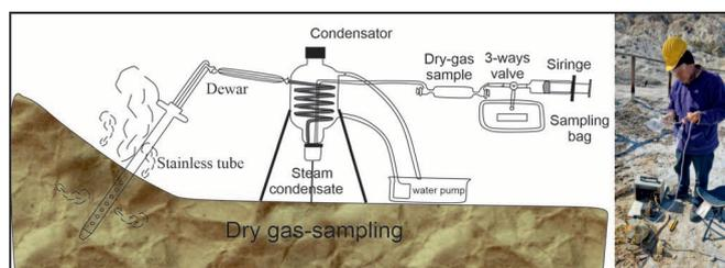
**Figure 3** Scheme for sampling gas from fumaroles; on the right, operations at the Solfatara crater.
