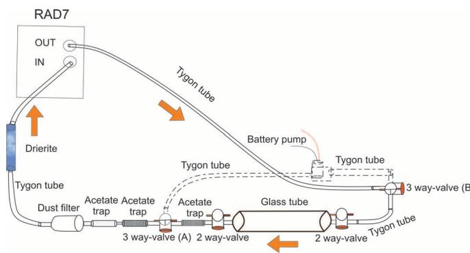
**Figure 8** Configuration for connecting the glass tube to RAD7 to measure radon gas sampled from fumaroles. Arrows indicate the direction of gas flow. The dashed part is excluded from the flow path.
