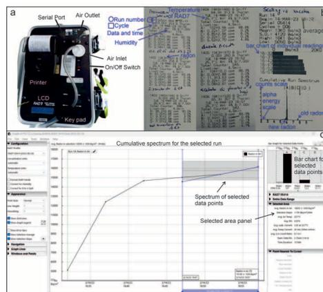
**Figure 1a** RAD7 instrument. Note the inlet and outlet valves for gas; **1b** example of printouts with explanation of the significant parameters; **1c** example of Capture graph with radon content in air gas at each recycle. The dashed area is related to the last three stable measurements.
