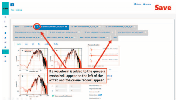
Figure 26 When a waveform is added to the queue, a new tab will appear after the other waveforms' panel.
