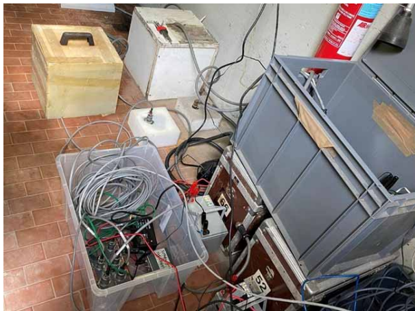
Figura 13 Stazione sismica TV.TEST posizionata accanto alla stazione IV.MILN: a) REFTEK Wrangler-HDR; b) Trillium Compact Horizon 120s; c) Episensor FBA ES-T; d) GAIIV; e) Trillium 40s; f) Episensor FBA ES-T. Figure 13 Seismic station TV.TEST located next to station IV.MILN: a) REFTEK Wrangler-HDR; b) Trillium Compact Horizon 120s; c) Episensor FBA ES-T; d) GAIIV; e) Trillium 40s; f) Episensor FBA ES-T.
