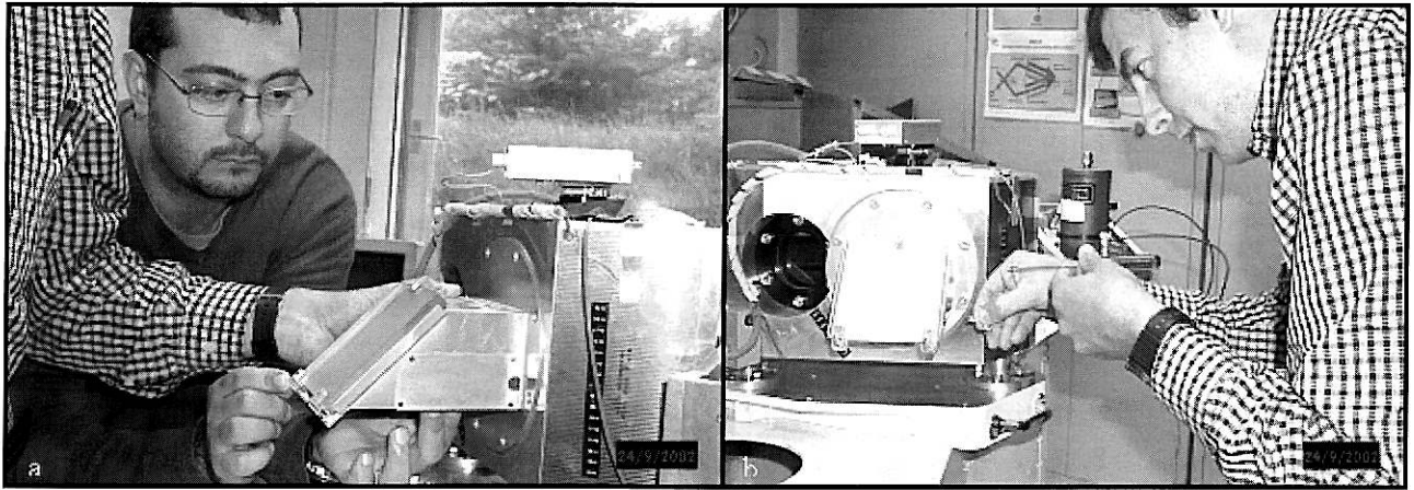
Fig.8: a) verification of the Germanium Flange and MIROR interface; b) Flange assembly.
