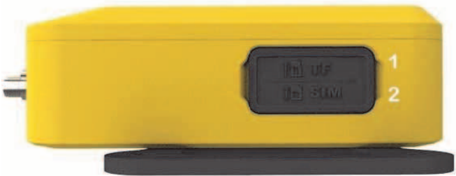
Figura 3 Dettaglio slot SIM e CF SC600+. Figure 3 SC600+ SIM and CF slot detail.
